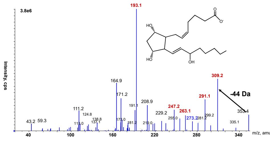
**Fragmentation scheme of PGF<sub>2</sub> $\alpha$  [M-H]<sup>-</sup> m/z 353**
